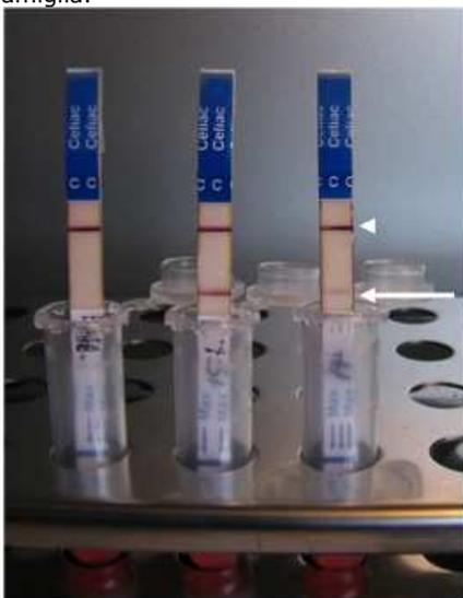
The first band (head-arrow) must always appear as technical control, the second band (arrow) represents the positive result of the test. No second band was detected in the first strip incubated with blood sample tested negative for anti-transglutaminase antibodies. Different shades of gray bands identified celiac patients in the second and third strip.
